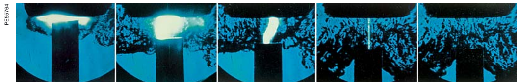
Electrical arc in a self-expansion breaking chamber
